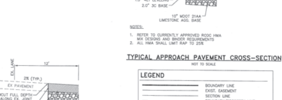
TYPICAL WIDENING PAVEMENT CROSS-SECTION NOT TO SCALE
