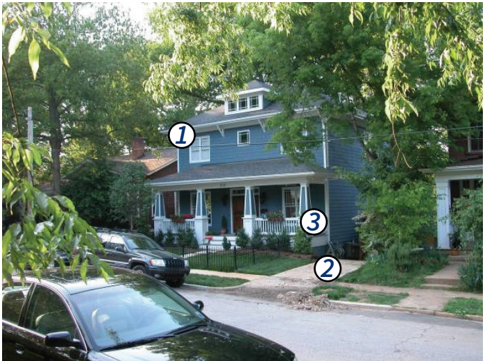
The examples above from Denver, Colorado, and Fredericksburg, Virginia, illustrate good examples of infill development within an established residential neighborhood. Both homes are designed using similar setbacks, building massing, and building heights to ensure compatibility with adjacent homes. And the homes use similar architectural features such as porches and columns.
