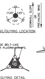
TREE STAKING DETAIL
