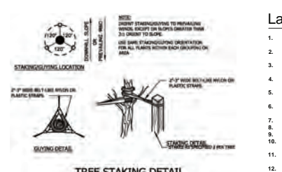
TREE STAKING DETAIL NOT TO SCALE
