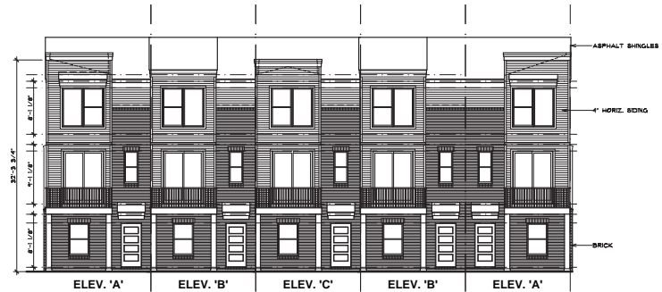
FRONT ELEVATION 5 UNIT BUILDING
