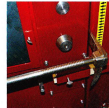
Outward forcing with latch bolt and 2x2 wood breaching
