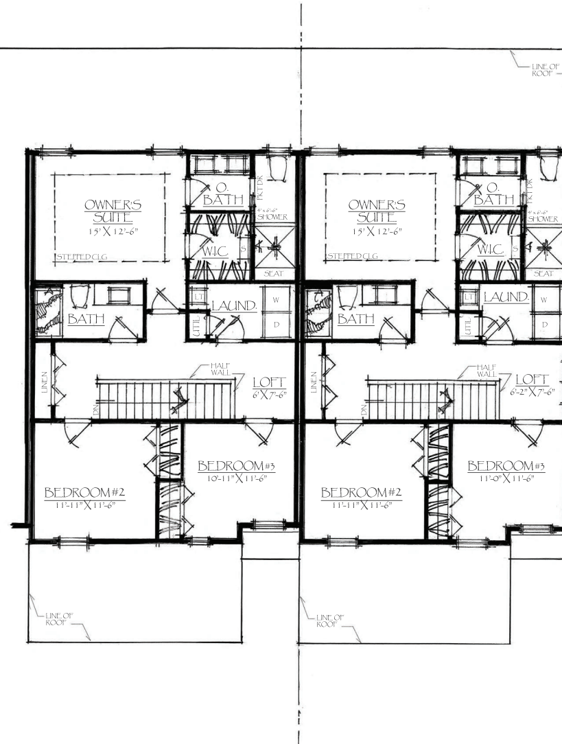
INTERIOR UNIT SECOND FLOOR SCALE: 1/4" = 1'-0"
