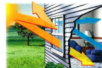
Summer Energy Savings: Low-E helps block unwanted solar heat penetration to help conserve air-conditioning use.
