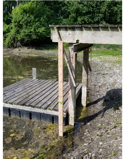
Water Level "gauge"
