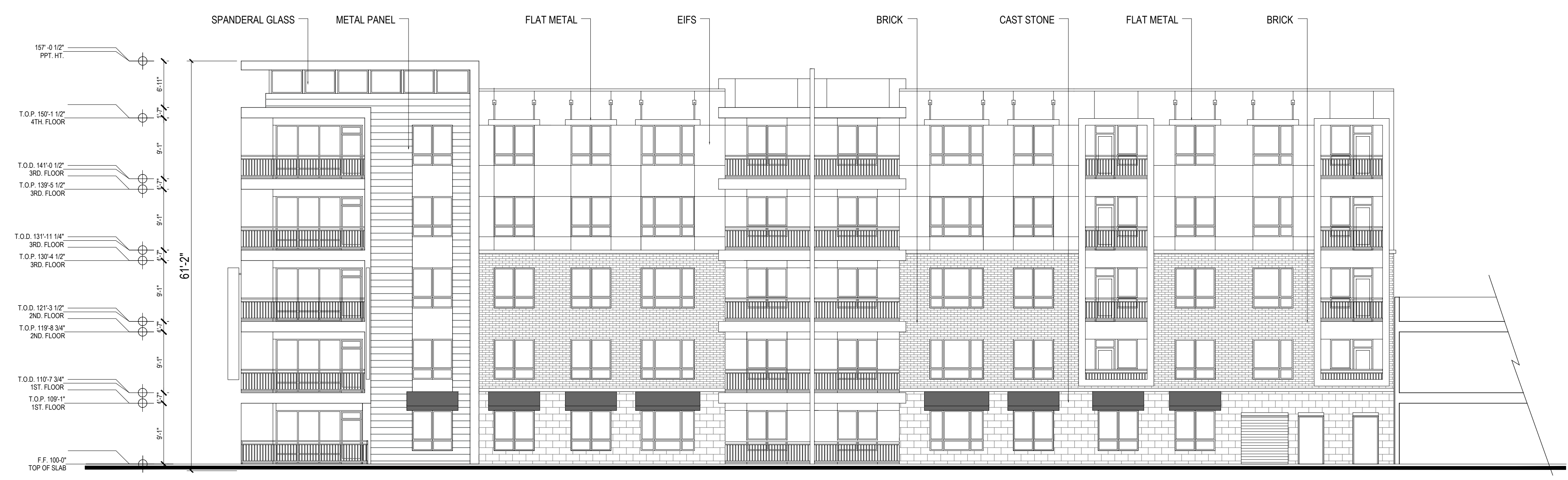
SIDE ELEVATION ( North )
