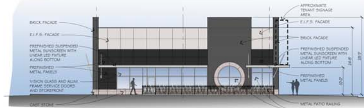
EAST ELEVATION SCALE: 3/32" = 1'-0" P4.4
