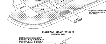
SIDEWALK RAMP TYPE C (CONTINUATION RAMP)
