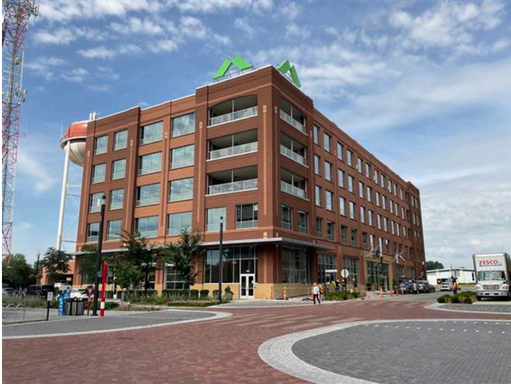
Merchant's Mortgage/Merchants Capital Corp offices. Variations in brick paving on the street denote driving lanes, crosswalks, "curb" and pedestrian realm without changes in grade or painting.
