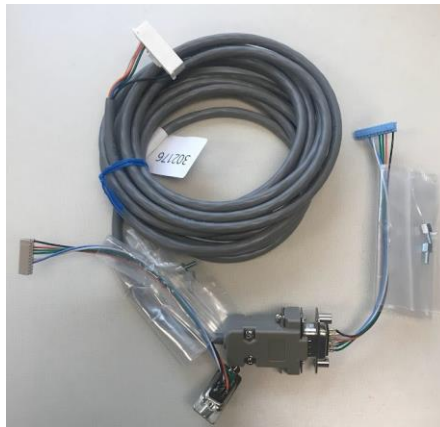
2nd Floor Coin Box Special Jamex cable to connect the Coin Box to our Canon Copiers
