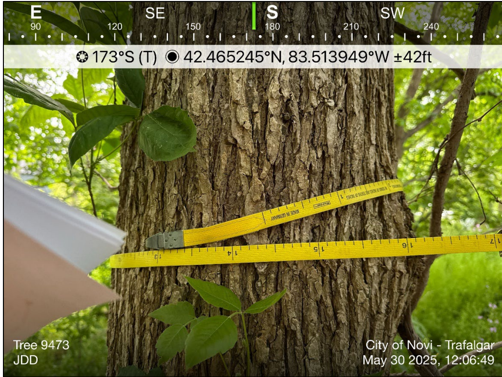
Overview of Tree 9473 with small difference in DBH Measurement with DBH tape vs. tree survey. Differences can occur between different measurement devices such as Biltmore stick vs. calipers vs. DBH tape
