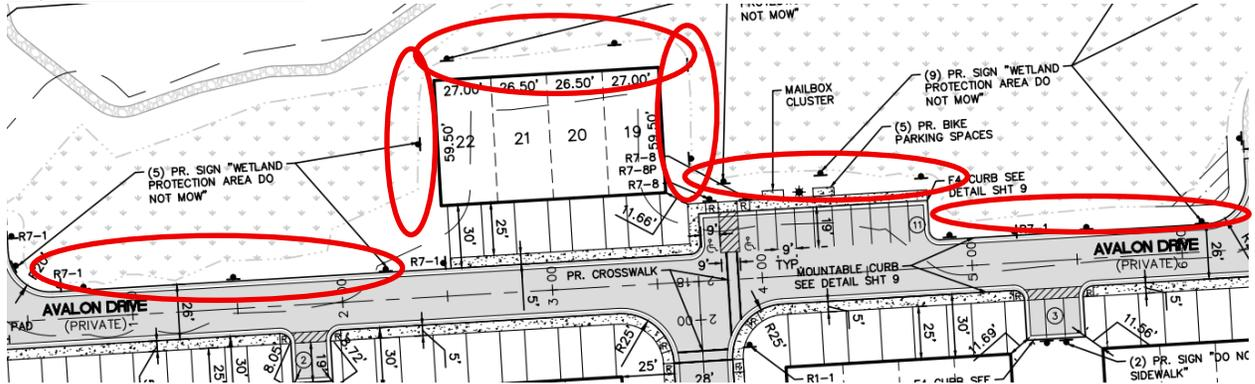
6. Portions of the wetland may become disconnected by the placement of fill throughout the site. It is requested that wetland equalizer culverts or similar structures be placed beneath roads that allow the wetlands on-site to remain connected. Specifically in the locations circled below. The eastern circled area reflects the approximate off-site portions of the wetland as delineated by ASTI on April 30, 2025.
