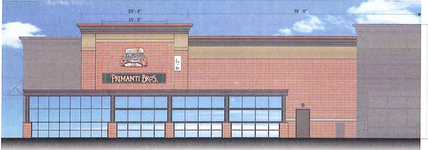
2 REAR ELEVATION (WEST): ID WALL SIGN FABRICATED ALUMINUM CABINET WITH 15MM RED NEON ILLUMINATION
