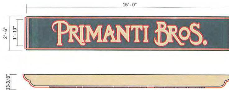
2 DETAIL: ID WALL SIGN FABRICATED ALUMINUM CABINET WITH 15MM RED NEON ILLUMINATION
