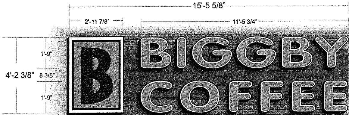
CHANNEL LETTER DETAIL SCALE: 1/2" = 1'-0"
