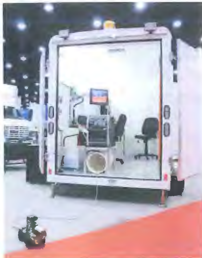
Optional reel stand, equipment wash down system, and rear monitor pictured above.
