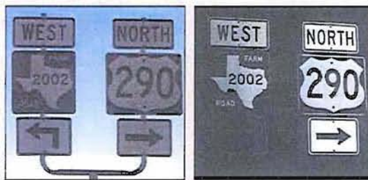
Retroreflective sheeting degrades over time. Daytime visual inspections cannot be used to assess retroreflectivity.
