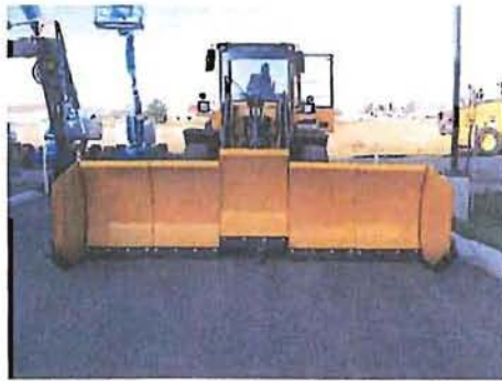
Box blade mounted on front-end loader
